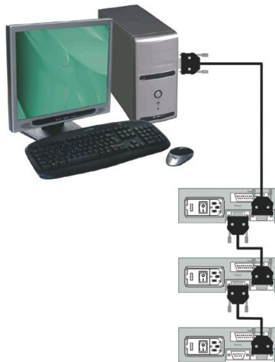
Figure 12. Example of connection of 3 boxes.
